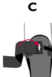
Place rubber molded end of strap over the Thumb Screw.
